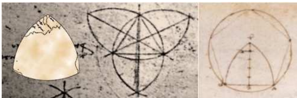
Figure 9. Details of pages from Leonardo da Vinci's notebook developing the geometry of his octant triangle figure, which was later developed as the Reuleaux triangle [ xiii ] (Leonardo da Vinci, Paris Manuscript A , 15v; Codex Atlanticus , 923r).
