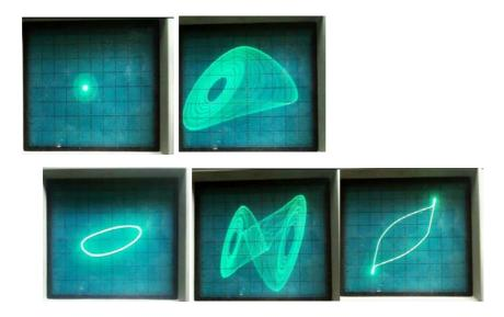
**Figure 10**. **Top Left** R=2.1 K Ohms. Single State Stability Point Attractor. **Bottom Left** R= 1.82 Ohms, Harmonic Oscillation between V1 and V2 (Lissajous pattern).
